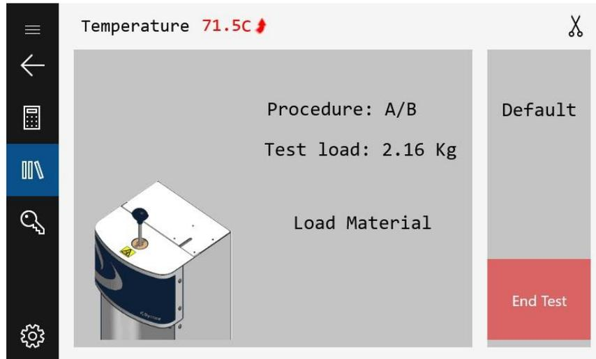
After loading the material, press the screen. The LMI will prompt you to insert the piston and add the weight to the LMI. The encoder arm must also be placed underneath the weight.
