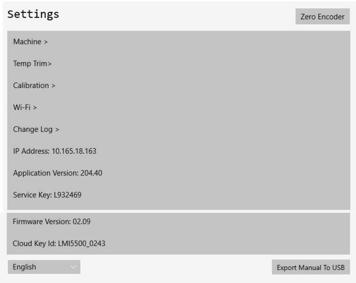
**Zero Encoder Button** – Re-zeros encoder position in the event that the machine was started without the encoder in the correct position. If encoder reset is needed, put the encoder in the fully down position and press this button to reset the position.
