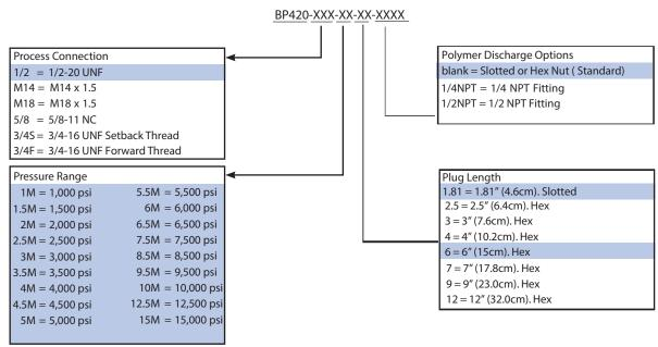
Shaded sections refer to standard (short lead time) configurations. Consult the factory for other configurations that may be available.
