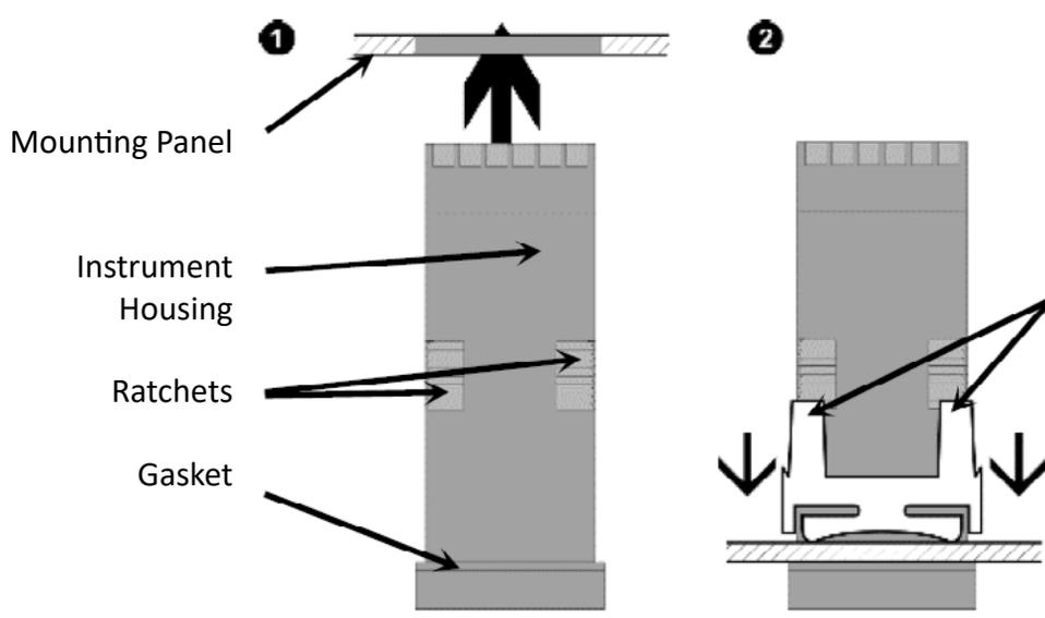
1. Insert instrument into the panel cut-out.
